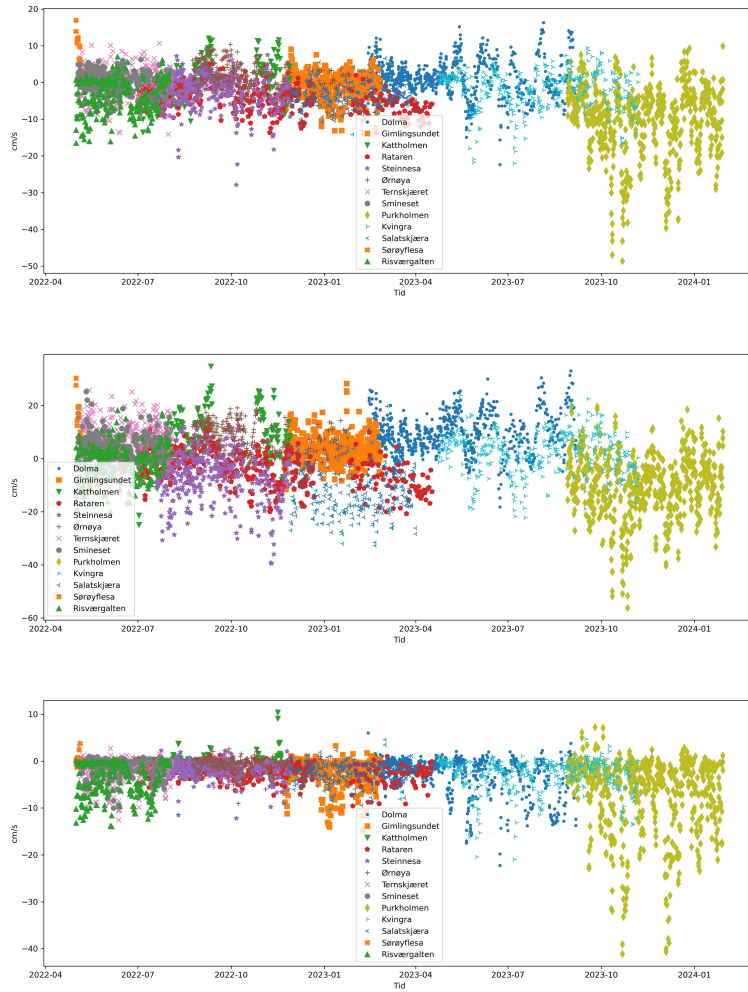
Figure 4.4: Time evolution of the difference between measured and modeled daily median speed (top) maximum speed (middle) and minimum speed (bottom). Data from all times and depths were included. The color and symbol of a point indicate the measurement site.
